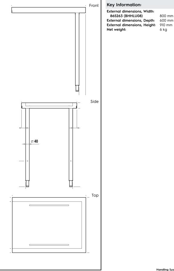
Handling System for Hood type Dishwasher Table Unloading/Loading, 800mm
